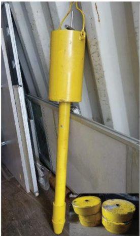
图 2 重力取样器模型、配重块 Fig.2 Model of gravity piston corer and counterweight
